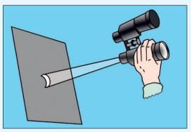
A pair of binoculars can stand in for a pinhole. Cover one eyepiece with the lens cap, then when the binoculars are pointed at the Sun you should see its image projected onto the plain card. Use the focus wheel to sharpen the image. This method works best if both the card and binoculars are mounted on a tripod.
