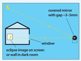
and mirror size should make the image brighter. To make the image clearer to see, use an indoor wall in a house and reflect the image in through a window.
